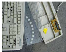
Sensors of keys in a computer keyboard
