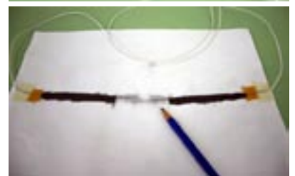
Image of Wiring prototype for the drawn switch. Wiring recognizes the resistance in the graphite line between two copper lines.
