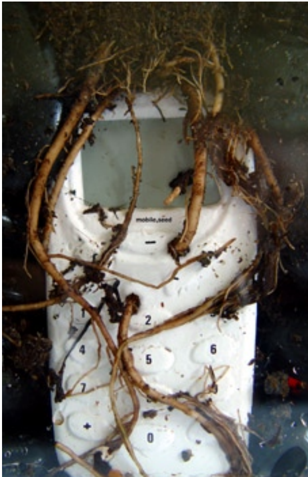
Fig. 4.37 A prototype made with biodegradable biopolymer made from starch. The roots of the flower nourishes from the decomposition of the material.
