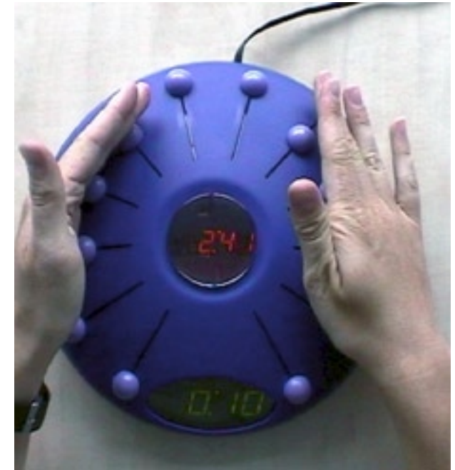
Fig. 2.2 Aesthetics of the interaction. Prototype of alarm clock. When sliders are slid from the starting situation towards the central display, the alarm time changes.
