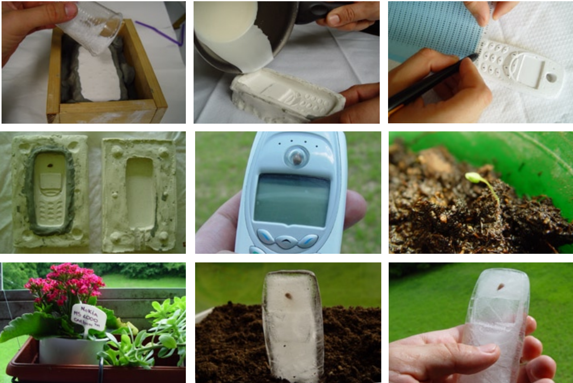
Fig. 4.45 Images from prototypes and tests made for the communication of the Mobile.Seed project, using plaster, silicon, rubber and ice.
